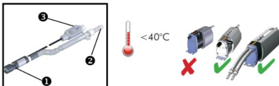
Insert the sensor **❶** into the condensate tray pipe as shown and secure the hose **❷** in position. The DrainStik® must be mounted vertically. Use the silicon hose provided.
