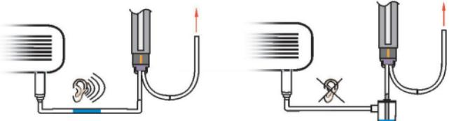
If the pump is installed remotely, occasionally water can become trapped in the u-bend at the lowest point of the system. Due to the pump's high flow rate, this can create a gurgling noise.
