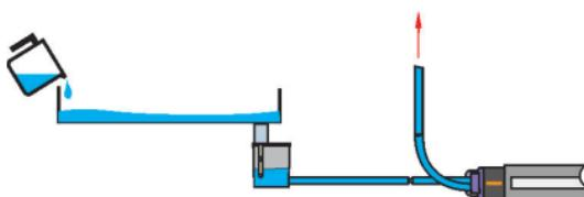
The water test ensures that the pump responds to the water level & that the pump switches off when dry. To test, slowly pour cold water into the tray until the pump switches on. Allow the pump to run and switch off. The pump should run for approximately 20 seconds after emptying the reservoir/condensate tray pipe.
