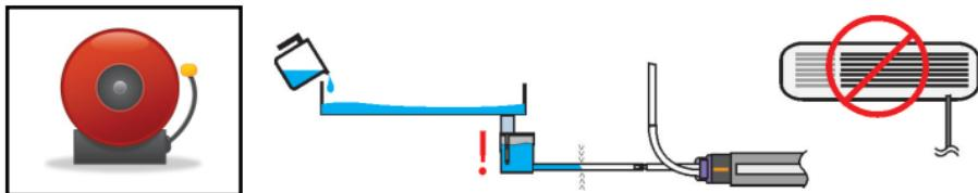
To ensure that the alarm connection is working, restrict the outlet of the reservoir/DrainStik™ hose and fill with water up to the high level sensor. The pump will turn on initially, then after a short delay the alarm relay will switch, detected using a multimeter or observing the shut down of the AC unit. Allow the water to exit the reservoir; the water should then be pumped away, and AC operation will restart.
